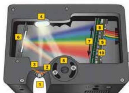
Fig.2 Inside schematics of the integrated spectrometer
